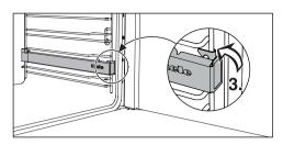
■ Then secure the FlexiClip runner to the bottom of the two rails as illustrated (3).
